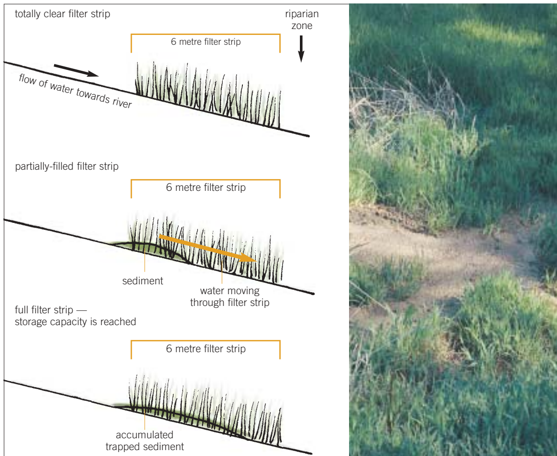
How a filter strip works. Illustration Carolyn Brooks. Photo Ian Prosser.
