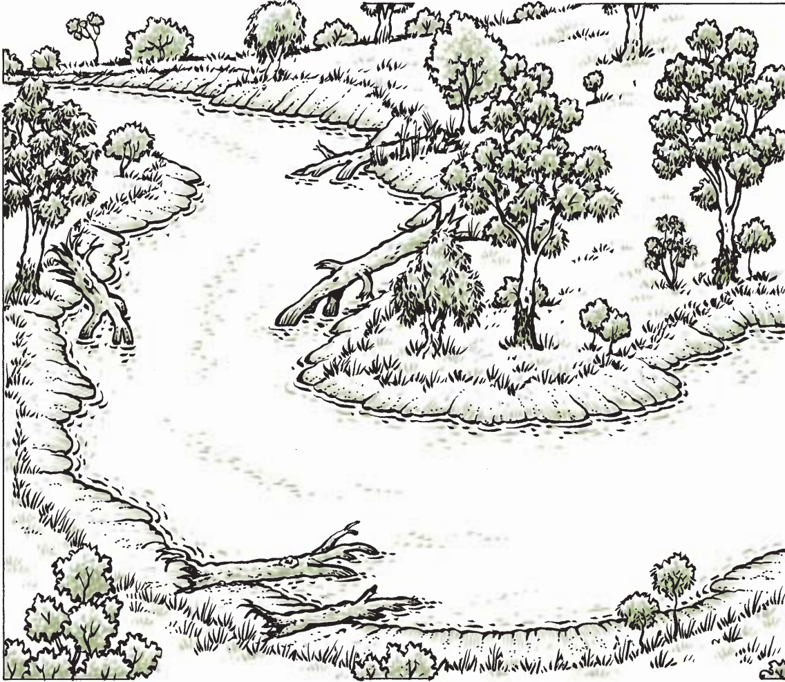
Large snags repositioned if necessary to minimise their possible effects on flow downstream or onto the bank (flow is from upper left to lower right). Illustration Paul Lennon.
