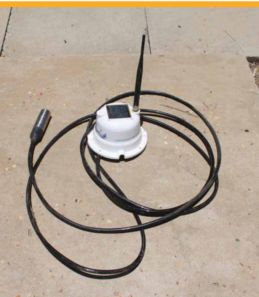
Figure 2: The tank sender is located on top of the tank and transmits a signal to the receiver.
