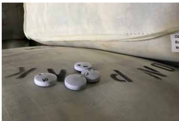
Digibale bluetooth beacons used to monitor temperature and humidity of the wool in wool bales during transport (Source: Department of Jobs, Precincts and Regions).
