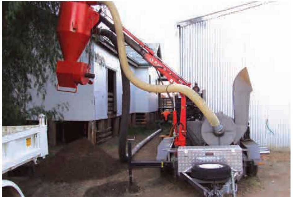
The VacTrax vacuum cleaning machine is able to suck out manure from under shearing sheds quicker and much easier than traditional methods.
