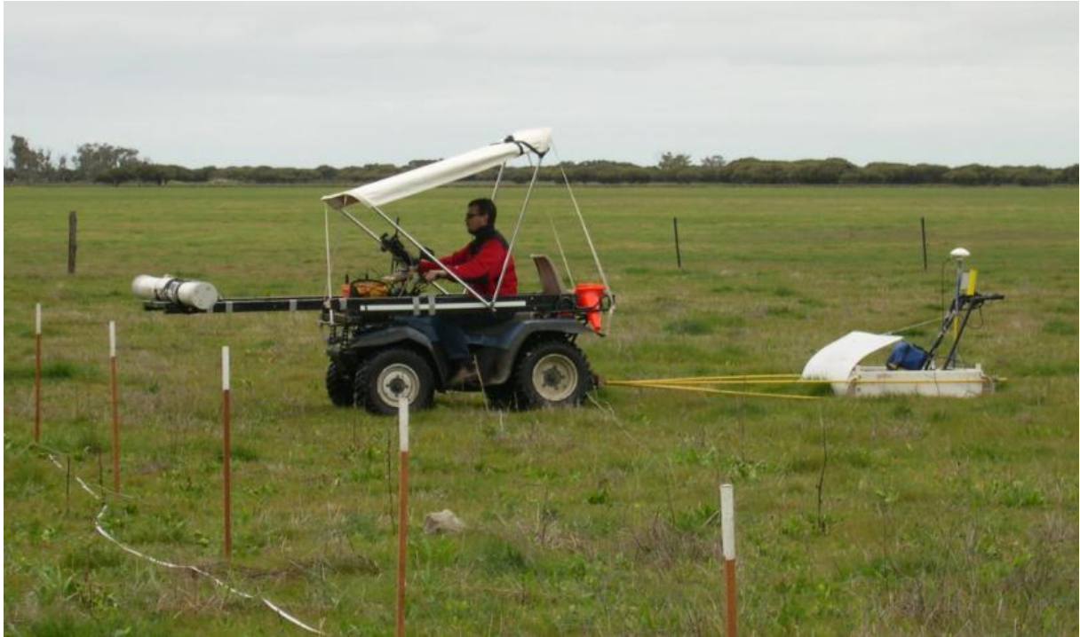
Figure 9: Ground penetrating radar and EM31/38 survey being conducted on the authors property. (Source: Author, 2006)
