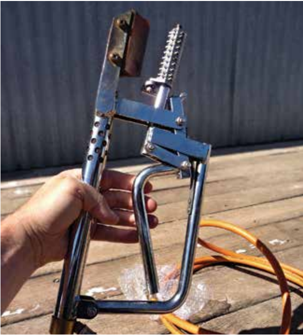
Figure 3.2: The Te Pari Patesco knife with a rotating anvil
