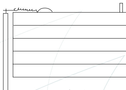
Figure 2 The Spring attached to the gate
