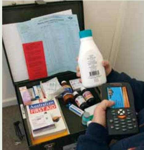
Figure 1 Scanning the barcodes of products in the medical chest using the personal digital assistant.
