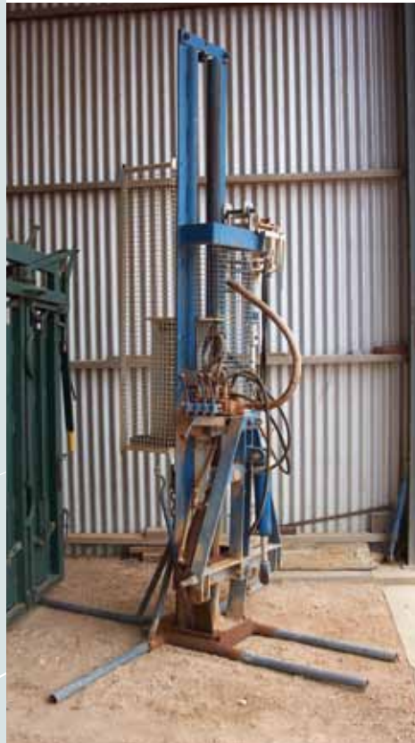
Figure 1 The frame allows the digger to stand independently
