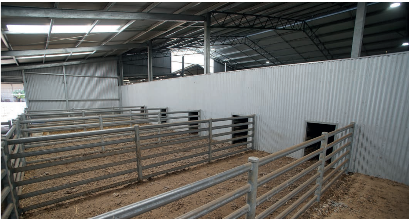
Count-out pens are under cover and are also used as additional yarding. A ramp to the right of the picture allows sheep up onto the raceway behind the catching pens.
