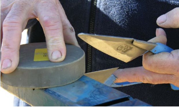
Photo 5.56 Gently push the blade into the chosen slot until the sharpening edge just pushes the stone slightly upwards. PHOTO: Ian Evans
