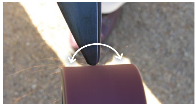
Photo 5.52 Grinding the points on 'closed-point' shears. For 'open-point' shears grind each point individually. PHOTOS: Ian Evans
