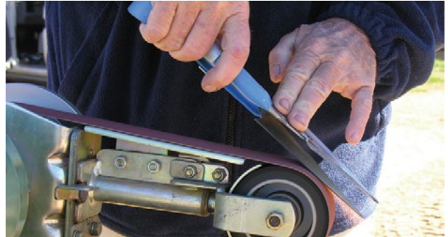
Photo 5.49 Without using too much pressure guide the blade across the grinding wheel 3–5 times. PHOTO: Ian Evans
