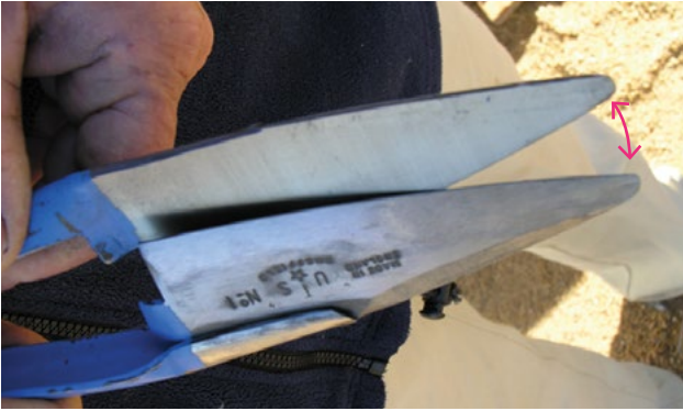
Photo 5.62 Backing off from point (top) to heel (bottom). PHOTOS: Ian Evans
