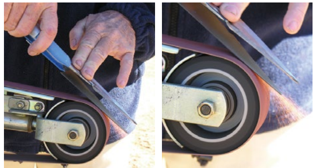
Photo 5.50 Start grinding from the heel of the shears. PHOTOS: Ian Evans
