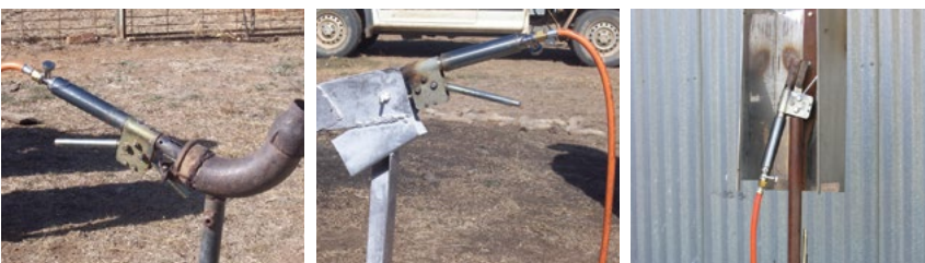
Photo 5.68 A range of gas-knife holders illustrating varying degrees of safety. PHOTOS: Ian Evans
