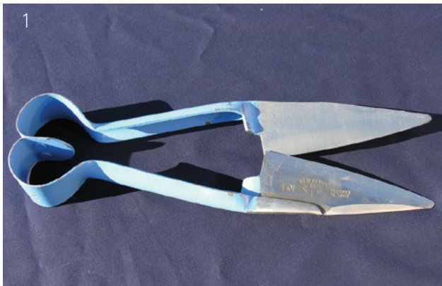
Photo 5.33 Ideal set occurs when the top blade just comes across the bottom blade when released to a relaxed position. PHOTO: Ian Evans
