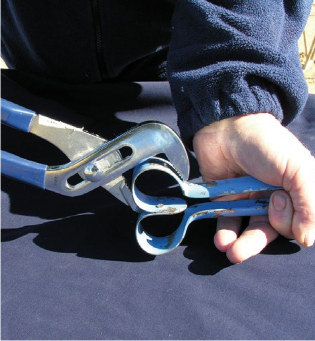
Photo 5.31 Close and hold the shears past the knockers, as previously shown, and using a large pair of multi-grips, grip each bow as shown below and gently squeeze each bow in turn. PHOTO: Ian Evans
