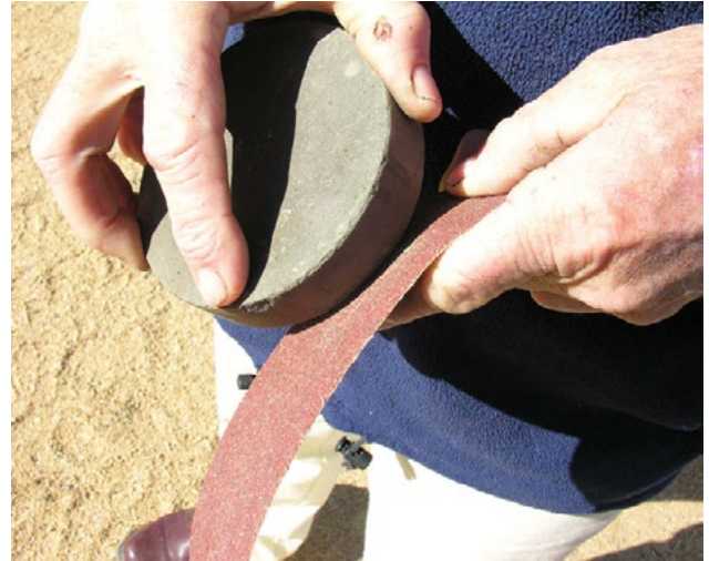
Photo 5.54 The edges of sharpening stones can be bevelled by rubbing on an old grinding belt (above) or a concrete surface (right). PHOTO: Ian Evans
