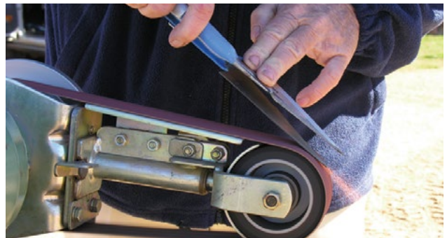
Photo 5.51 Draw the blade all the way through to the point. PHOTO: Ian Evans
