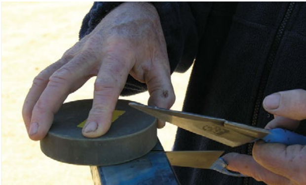
Photo 5.59 Rub the sharpening face of the blade, using a circular motion. PHOTO: Ian Evans
