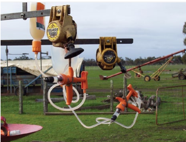
Photo 5.76 Unique recoiling suspension system for vaccination guns. Excellent for operator safety, hygiene and efficiency of use.
