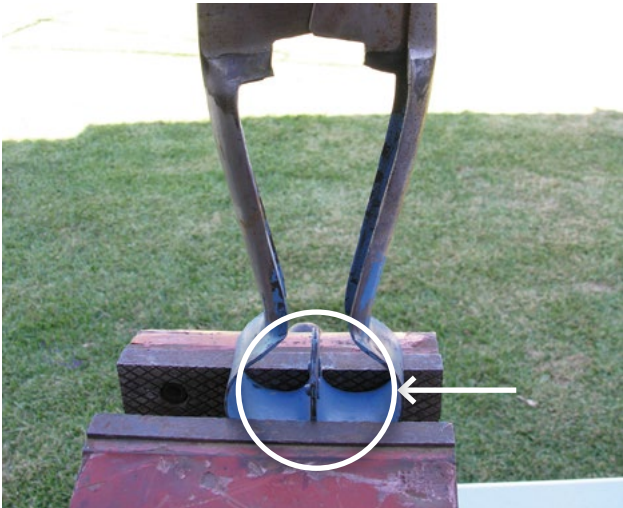
Photo 5.24 Hold the bottom 10-20mm of the shear bows in a vice. Do not over-tighten the vice and crush or deform the bows. PHOTO: Ian Evans
