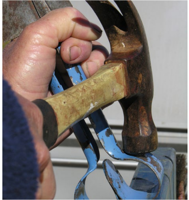
Photo 5.30 Holding the shear closed turn it over and repeat the gentle hits on the other side. PHOTO: Ian Evans
