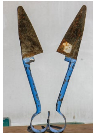
Photo 5.11 Too wide at heels – too much tension in the bows. PHOTOS: Ian Evans
