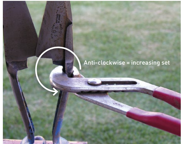
Photo 5.25 Use a large pair of multi-grips just below the knocker. To open the set (increase the clearance at the heel), gently twist the handle anti-clockwise. To close the set, decrease the clearance at the heel and gently twist the handle clockwise. PHOTO: Ian Evans
