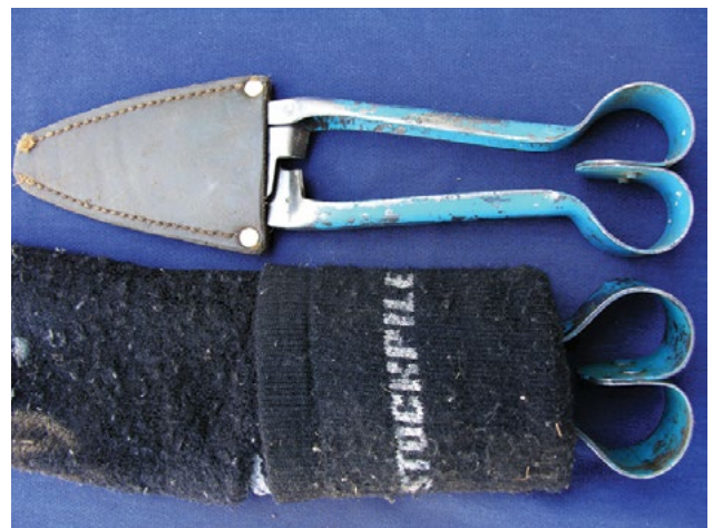
Photo 5.65 Leather sheaths (top) can cause condensation, promote rust and damage the set. It is better to store blades in a woollen cover (bottom and below). PHOTOS: Ian Evans
