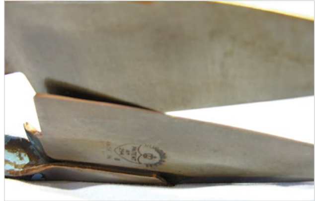
Photo 5.16 When shears are fully opened there should be one point of light contact between the blades. PHOTO: Ian Evans
