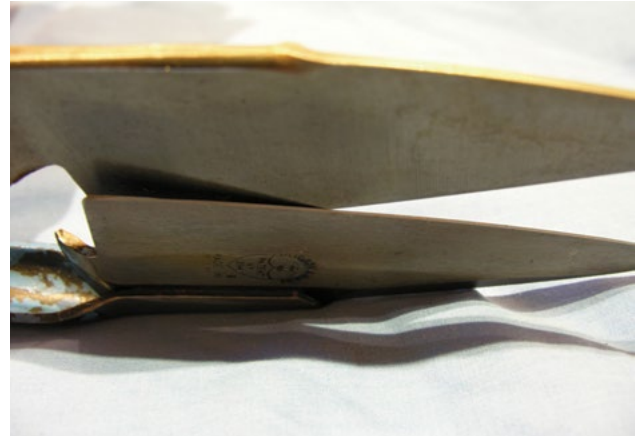
Photo 5.23 For an effective cutting action, the blades must lean towards each other so the cutting edges touch at only one point at a time. PHOTO: Ian Evans
