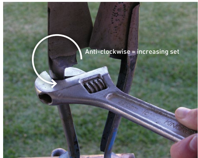
Photo 5.26 A 'shifter' or adjustable wrench can be used instead of multi-grips. PHOTO: Ian Evans
