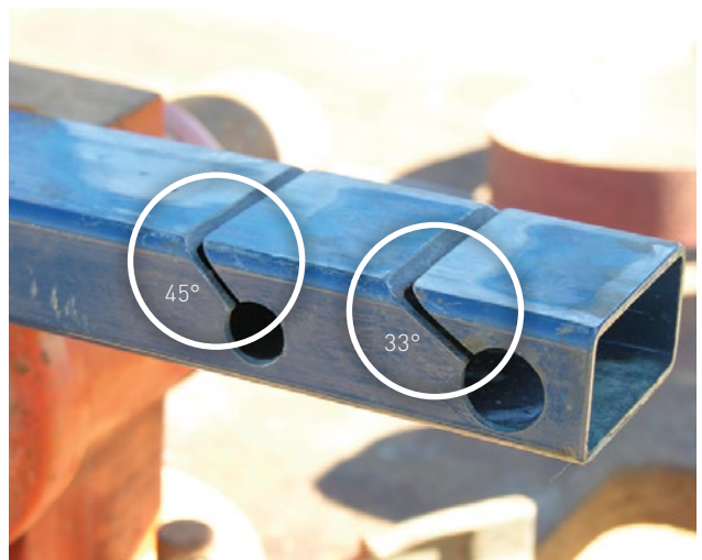
Photo 5.55 Some jigs have provision for sharpening at different angles. For example 45° (left) and 33° (right) in both of these images. PHOTOS: Ian Evans
