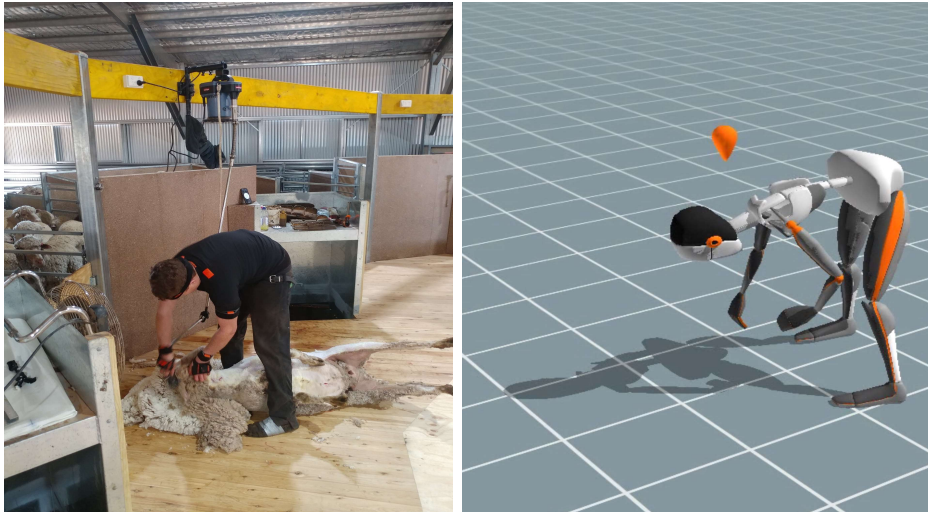
Figure 1. The portable data collection system that captured the motion and muscle activities of the shearer.
