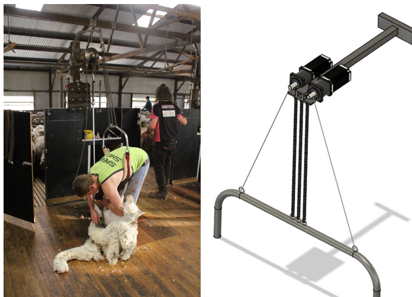
Figure 5. Shearer support back-harness (left). Concept of a modification to provide additional active support using a simple cable robot driven from above by electric motors (right).
